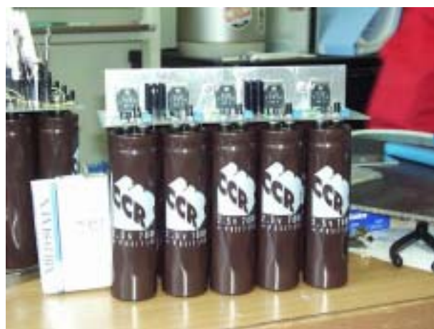
Fig.8 EDLC bank using organic electrolytic solution (1999-2000).
